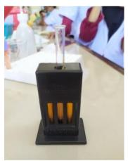
added CuSo4 solution 1% as much as 2 ml and NaOH 1% as much as 2 ml where cuso4 solution and NaOH solution is used to see the discoloration.
